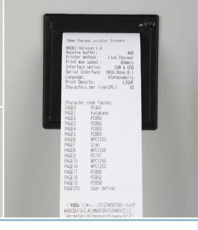
Maxim PNP-5850 is loaded from the front and is well suited for manned applications where trained staff use a device or instrument. It is regularly used in building control panels, diagnostic equipment, medical devices, measuring instruments and much more. PNP-5850 features a closed body with a rugged clamping system specially made for sustaining high vibration situations. It also features a dual data input system consisting of USB and serial ports.
